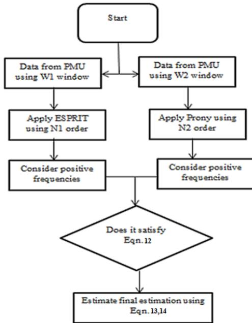
Figure 2. Block diagram representation of the proposed algorithm
