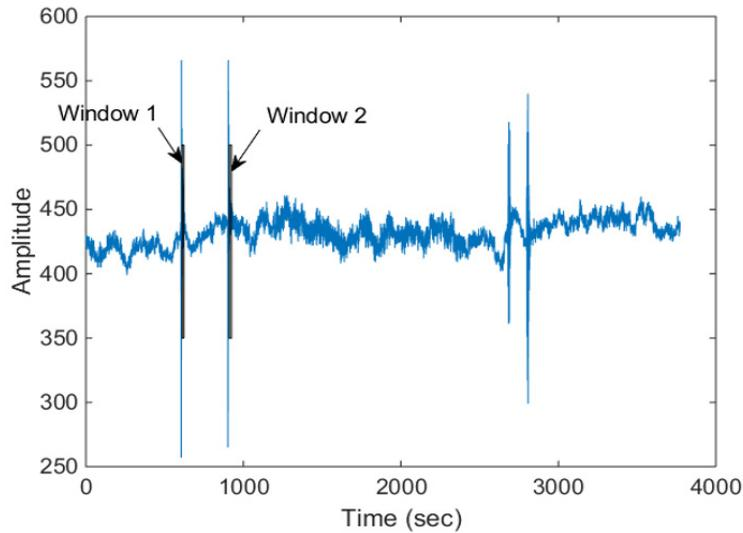
Figure 7. Test probe data of WECC system on 14<sup>th</sup> September 2005 with consideration of two windows to be analyzed.
